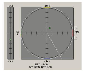
In the example above, the center of the graph is our standard, and the green dot is the sample. The sample is darker (-L), redder (+a), and yellower (+b) than the standard. The total color difference is summed up as DE\* = 0.34 with the white circle being the tolerance of 1.00 DE\*. This sample passes tolerance.
